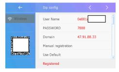
If the domain is still different, touch the address to bring up a keypad and manually enter 47.91.88.33.
