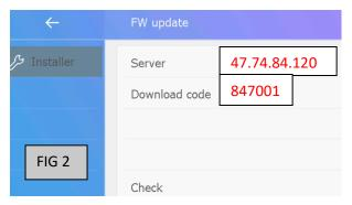
From the home screen select: Settings, installer, right arrow up the top right of screen, FW upgrade. Change the settings to FIG2 then check for upgrade, if available, select INSTALL. This may take a while depending on your internet connection speeds and any port forwarding issues imposed by your router so please be patient.
